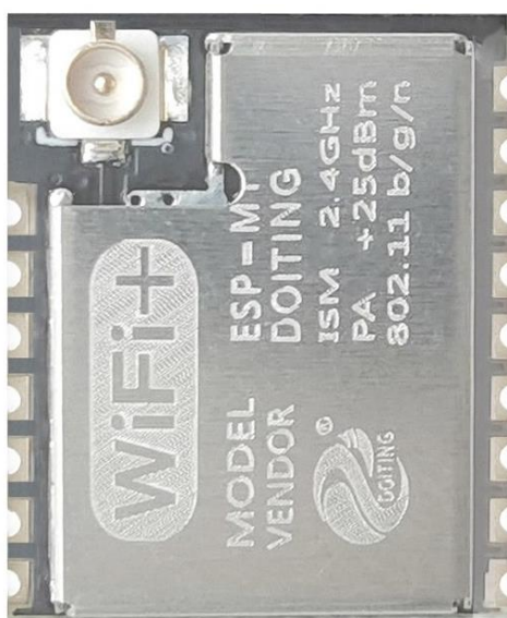
Fig.3.1 Shape for ESP-M1
