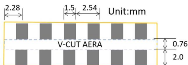
Fig. 3.3 PCB Layout for ESP-M4
